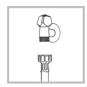
1. Connect the supply pipe by screwing it to a cold water tab using a ¾ gas threaded connection (see figure). Before performing the connection, allow the
